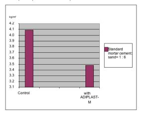
Hydrophobication, water absorption at 24 hours
